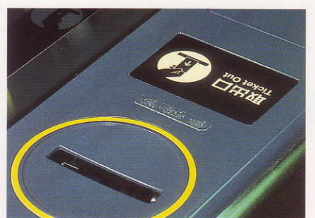
▲ Ticket pick-up slot of automatic gate (with yellow indicated frame and braille plate) • 自动售票机的取票口 (镶边、盲文)
