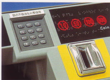
▲ Customer operation unit on ticket vending machine (with ten-key and braille guidance) • 售票机乘客操作部分 (键盘、盲文)
