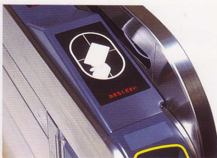
▲ Ticket insertion slot of automatic gate (with yellow indicated frame and braille plate) • 自动售票机的投票口 (镶边、盲文)
